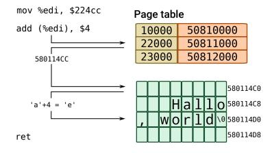
When second instance of a program will start, new process with separate address space will be created, thus making independent copy of process data, including "Hallo, world" message, but with same addresses. When process (actually its thread or task) is dispatched onto CPU, address of its page table is written to a special register (like CR3 on x86), so only it may access its data. All address translations are performed by *Memory Management Unit* in CPU and are transparent for it.
