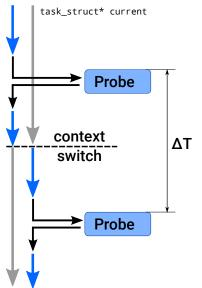
So if we count that timer probe has fired two times, once in context of left process and once in context of right process, we can conclude that they both consume 50% of CPU time, like prstat and top utilities do. Profiling will be covered in Profiling section of Module 3.
