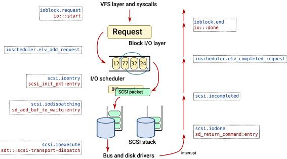
Both Solaris and Linux use SCSI protocol as unified way to represent low-level device access. SCSI devices can be stacked, i.e. with *device mapper* in Linux or *MPxIO* in Solaris, but we will have only single layer in our examples. In any case, this subsystem is called *SCSI stack*. All requests in SCSI stack are translated to SCSI packets (which can be translated to ATA commands or passed as is to SAS devices). SCSI packet is handled in a several steps:
