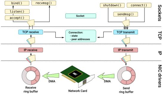
Network input-output can require transferring huge amounts of data, so it may be ineffective to explicitly send write commands for each packet. Instead of handling each packet individually, NIC and its driver maintain shared *ring buffer* where driver puts data while card uses *DMA* (direct memory access) mechanisms to read data and send it over network. Ring buffers are defined by two pointers: *head* and *tail*:
