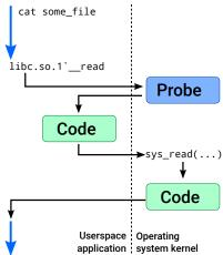
In DTrace userspace tracing is performed through pid provider:
