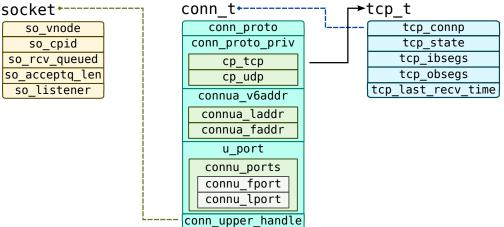
Solaris wraps sockets into sonode structure which are handled by virtual file system called *sockfs*. so\_vnode field in that structure points to VFS node. Like we mentioned before, TCP and UDP connection are managed by conn\_t structure. It keeps addresses in connualaddr and connu\_lport fields for local address and uses connua\_faddr and connu\_lport for remote ports. Note that these names are different in Solaris 10.
