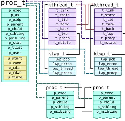
Current thread is passed as curthread built-in variable to probes. Solaris proc provider has lwpsinfo\_t and psinfo\_t providers that extract useful information from corresponding thread, process and LWP structures.
