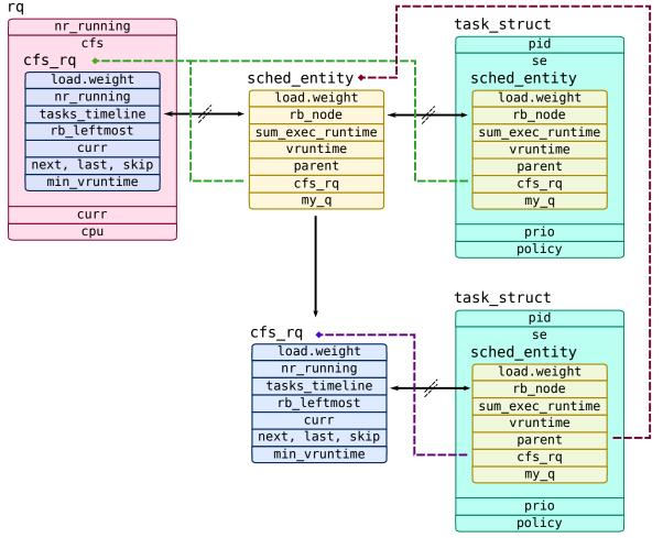
In this example processor run queue has two scheduler entities: one CFS queue with single task (which refers top-level cfs\_rq through parent pointer) in it and one top-level task.
