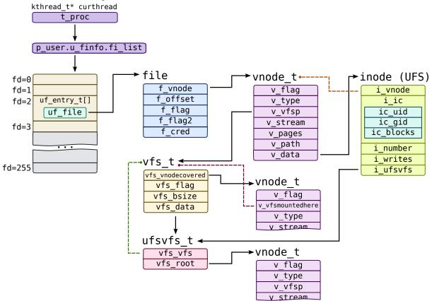
Like Linux, each process keep an array of uf\_entry\_t entries while entry in this array points to an open file through uf\_file pointer. Each file on filesystem is represented by vnode\_t structure (literally, *node on virtual file system*). When file is opened, Solaris creates new file object and saves open file mode in flag fields f\_flag and f\_flag2, current file position in f\_offset and pointer to a vnode\_t in f\_vnode.
