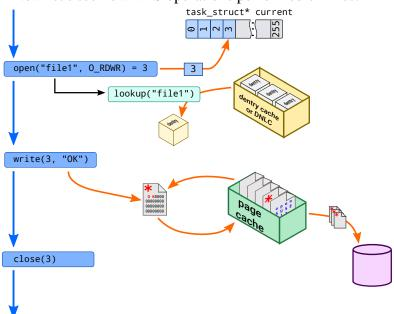
Application uses open() system call to open file. At this moment, new file object is created and free entry in open files table is filled with a pointer to that object. Kernel, however needs to find corresponding vnode/dentry object — it will also need to check some preliminary checks here. I.e. if uid of opening process is not equal to i\_uid provided by operating system and file mode is 0600, access should be forbidden.
