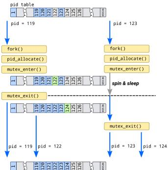
When process 119 acquires new process id, it leaves mutex by calling mutex\_exit(). This function activates other process, 123, which may now access pid table, but it can't get process id 122 because process 123 is already sees changes made by process 119. So it takes next available pid which is 124.
