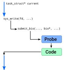
When process wants to start synchronous write, it issues write() system call and by doing that it transfers control to a kernel code, to a sys\_write() function in particular. This function eventually calls a submit\_bio() function which pushes data from user process to a queue of corresponding disk device. If we attach probes to these functions, we can gather the following information:
