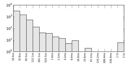
Y axis is logarithmic and represents a number of observed intervals when CPU was busy for time period shown on X axis. If we normalize this characteristic, we will get probability density function.
