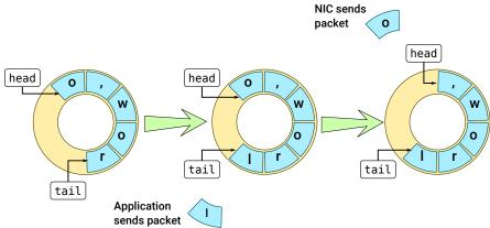
When driver wants to queue packet for transmission it puts it into memory area of designated ring buffer and updates *tail* pointer appropriately. When NIC transfers data over a network it will update *head* pointer.
