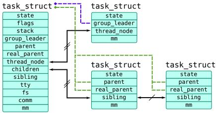
Task which is currently executed on CPU is accessible through current macro which actually calls function to get task from run-queue of CPU where it is called. To get current pointer in SystemTap, use task\_current(). You can also get pointer to a task\_struct using pid2task() function which accepts PID as its first argument. Task tapset provides several functions similar for functions used as Probe Context. They all get pointer to a task\_struct as their argument:
