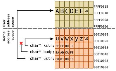
Accessing a data in kernel address space in DTrace is performed by simple dereferencing it in C-style. For example, fop\_open() function accepts pointer to pointer to vnode\_t, so to get actual address of vnode\_t, you need to dereference it:
